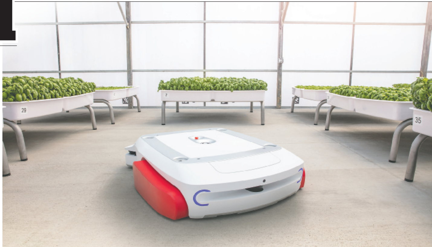
The “workhouse and backbone” of Iron Ox’s greenhouse automation system, mobile support robot Grover navigates through the greenhouse to get plant-growing modules wherever they need to be and is capable of lifting more than 1,000 pounds
