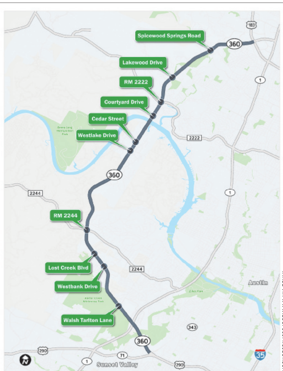
TxDOT's Loop 360 Program seeks to upgrade multiple intersections along the 14-mile corridor by removing traffic signals from the mainlanes and constructing overpasses or underpasses at select intersections. Additionally, shared-use paths for pedestrians and bicyclists will be added along Loop 360.
