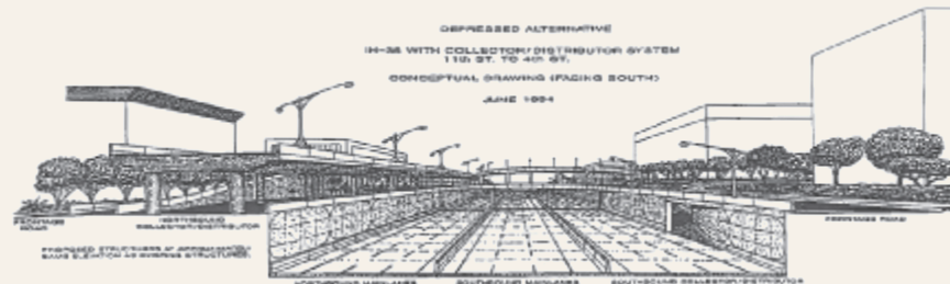
A proposed cross-section from the 1994 I-35 design concepts, showing the mainlanes (including HOV or “managed” lanes) depressed beneath the frontage roads and the adjoining city streets. Compare this to ...
