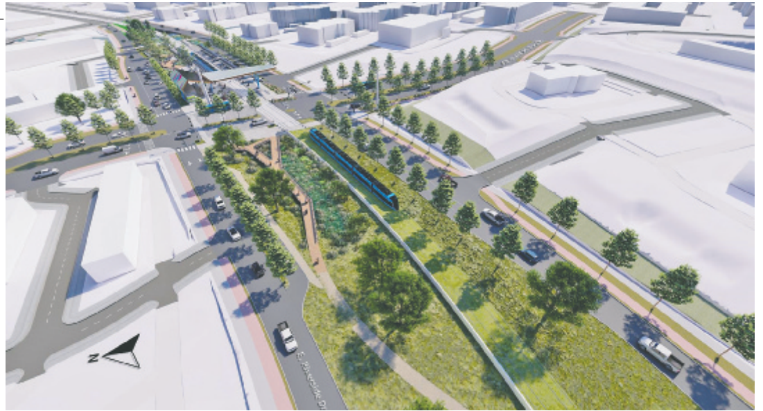
This aerial view (from the west) of the planned Riverside and Pleasant Valley station shows how the terrain slopes in both directions – including through the extra-wide right-of-way of East Riverside – which is a challenge when planning a transit hub that needs to be accessible to riders of all abilities.
