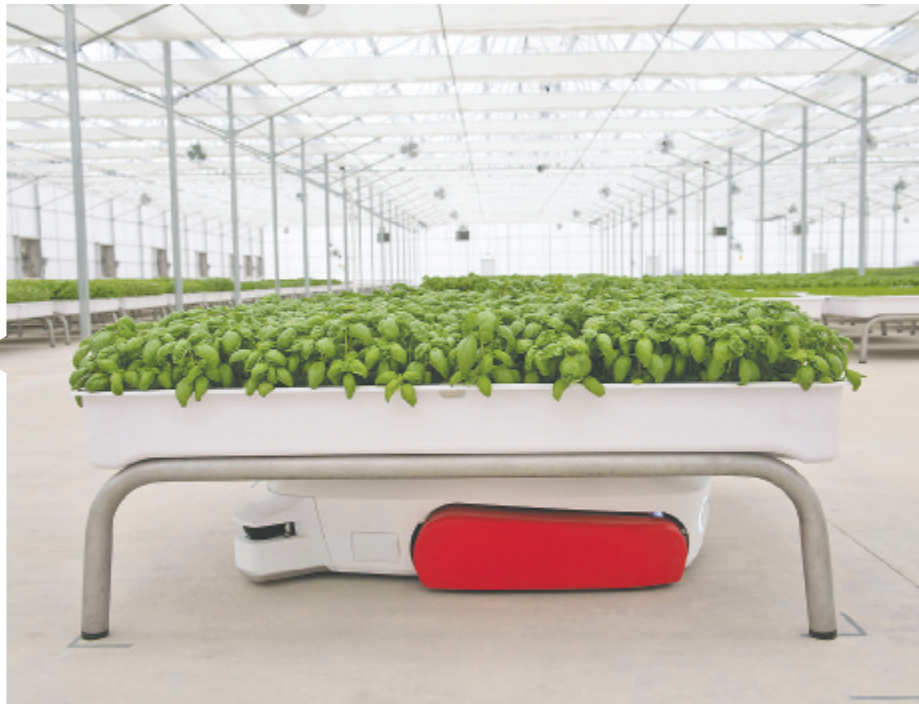
Mobile robots ferry plant modules, like this basil, to nutrient-rich watering stations tailored to each unique crop. This technology allows different crops to grow in the same greenhouse.
